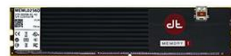
2. Diablo Technologies' all-flash Memory1 DIMM finds a home in a DDR4 memory slot.
