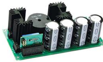
5. IXYS's Digital Inrush Controller incorporates an MCU module (a) and a main power board, shown here with MCU module (b).
