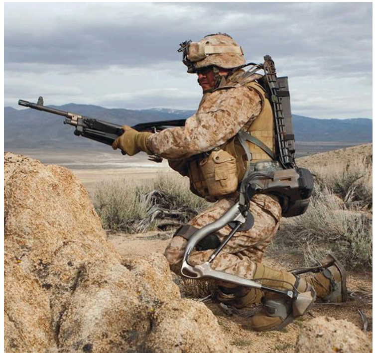
3. The HULC (Human Universal Load Carrier) uses hydraulics to provide heavy lifting capabilities.
